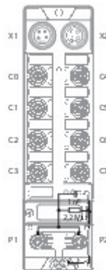
Fig. 10: TBEN-L4-8IOLA – equivalent wiring diagram and shielding concept
