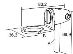
Filettatura vite: SMB30FA, A= 3/8 - 16 x 2 in; SMB30FAM10, A= M10 - 1.5 x 50
