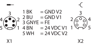
Fig. 13: Pin assignment voltage supply connectors
